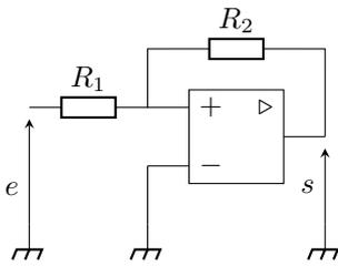
$$\triangleright \text{LNP} : \frac{e - v_+}{R_1} + \frac{s - v_+}{R_2} = 0 \implies \left( \frac{1}{R_1} + \frac{1}{R_2} \right) \varepsilon = \frac{e}{R_1} + \frac{s}{R_2} \text{ car } \varepsilon = v_+ - 0$$
