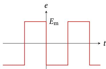
$$\begin{aligned} e(t) &= \frac{4E_m}{\pi} \left[ \sin(\Omega t) - \frac{1}{3} \sin(3\Omega t) + \frac{1}{5} \sin(5\Omega t) - \frac{1}{7} \sin(7\Omega t) + \dots \right] \\ &= \frac{4E_m}{\pi} \sum_{p=1}^{+\infty} \frac{(-1)^{p+1}}{2p+1} \sin((2p+1)\Omega t) \end{aligned}$$
